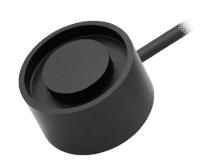
Ultrasonic transducer design covers 2MHz frequency. The sensor is paired with software as a signal sending and receiving unit. Used with a gel pad (or dry coupling), this sensor is particularly suitable for use as a non-invasive bottom-up liquid level sensor for measuring liquid level in plastic containers or vessels.
