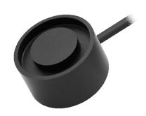
Ultrasonic transducer design 1MH<sub>7</sub> covers frequency. The sensor is paired with software as a signal sending and receiving unit. Used with a gel pad (or dry coupling), this sensor is particularly suitable for use as a non-invasive bottom-up liquid level sensor for measuring liquid level in plastic containers or vessels.
