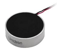
Ultrasonic transducer is designed to cover 1MHz frequency. The transducer works as a signal transmitting and receiving unit. The transducer works with gel pad (or dry coupling) is particularly for non-invasive bottom-up type liquid level sensors for measuring the level of liquid in a plastic container or vessel.
