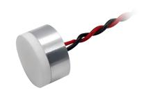
A200H1 ultrasonic transducer is designed to deliver outstanding performance at around 200 kHz frequency. The transducer works as a signal transmitting and receiving unit. This ultrasonic transducer is suitable for double feed detection, web guiding control and proximity measurement, etc.
