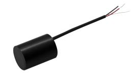
A200D1 works as a signal transmitting and receiving unit. This ultrasonic transducer is suitable for gas flow detection with high sensitivity, low noise, low ZFD (zero flow drift), high precision as well as exceptional reliability. In particular, the transducer housed with PVDF material is FDA compliance and free from corrosion by chemical solvent.
