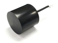
A050B1 works as a signal transmitting and receiving unit. This ultrasonic transducer is suitable for non-contact level detection and proximity measurement with extraordinary reliability. In particular, the transducer with the PVDF housing can operate under harsh chemical environment to measure the level of fluids, pastes, and coarse bulk materials.
