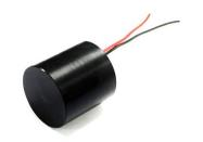
A125A works as a signal transmitting and receiving unit. This ultrasonic transducer is suitable for non-contact level detection and proximity measurement. In particular, the transducer with the PVDF housing can operate under harsh chemical environment to measure the level of fluids, pastes, and coarse bulk materials.
