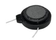
A500A ultrasonic transducer is designed to deliver outstanding performance at around 500 kHz frequency using our in-house piezoceramic and acoustic matching layer along with state-of-art technologies. The transducer works as a signal transmitting and receiving unit. This ultrasonic transducer is suitable for gas flow detection and proximity measurement with precise control as well as extraordinary reliability.
