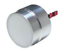
A220A ultrasonic transducer is designed to deliver outstanding performance at around 220 kHz frequency. The transducer works as a signal transmitting and receiving unit. This ultrasonic transducer is suitable for proximity measurement, web guiding control, non-contact level measurement and robotics, etc.
