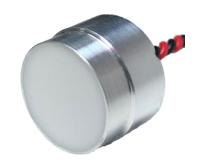
A150A ultrasonic transducer is designed to deliver outstanding performance at around 150 kHz frequency. The transducer works as a signal transmitting and receiving unit. This ultrasonic transducer is suitable for proximity measurement, web guiding control, non-contact level measurement and robotics, etc.
