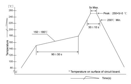
The products may be exposed to reflow soldering process of above profile up to two times
