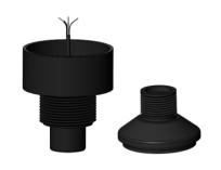
A125E works as a signal transmitting and receiving unit. This ultrasonic transducer is suitable for non-contact level detection and proximity measurement. In particular, the transducer with the PVDF housing can operate under harsh chemical environment to measure the level of fluids, pastes, and coarse bulk materials.
