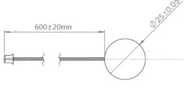
Drive Signal (VDriving): 1MHz 3.3v 20 pules, Drive interval: 10ms Echo Signal (VEcho): For 10cm olive oil level, echo signal appear around at 140us
