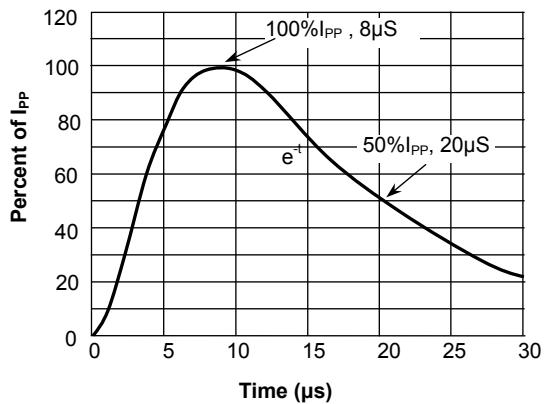
**Fig.4 Pulse Waveform-ESD(IEC61000-4-2)**
