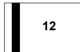
12 = Device Marking Code Bar denotes Cathode
