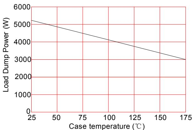
FIG.3: Load dump power characteristics
